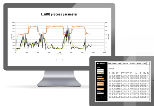
The L.ADU 260 provides drilling process data: Diagram with real-time data in digital form.
